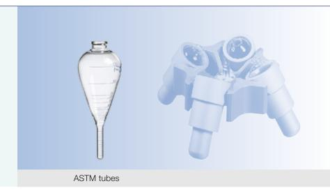
The sulphuric acid content of chrome baths can be determined by using chrome bath tubes. The method, which is intended to provide quality assurance information, is not only of interest to public and private test bodies, but also for the operators of the baths who wish to carry out the regularly necessary sulphate determinations themselves.
