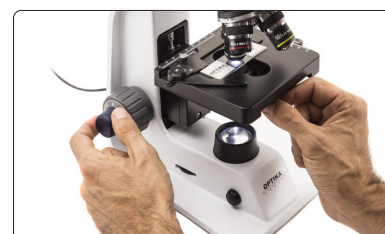
Regulation of diaphragm aperture
