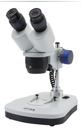
Cordless binocular stereomicroscope ideal for students, schools and amateurs to dissect and discover mainly biology and materials science in 3D, with turnable objective (2x-4x), FN 20 eyepieces, pillar stand and 1 W LED transmitted / incident illumination with rechargeable batteries. Slim and easy to carry, it is equipped with long lasting LED illumination to provide over 20 years of use
