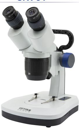
Cordless binocular stereomicroscope ideal for students, schools and amateurs to dissect and discover mainly biology and materials science in 3D, with turnable objective (2x-4x), FN 20 eyepieces, 360° rotating head, fixed arm with handle and 1 W LED transmitted / incident illumination with comfortable touch control and rechargeable batteries. Slim and easy to carry, it is equipped with long lasting LED illumination to provide over 20 years of use
